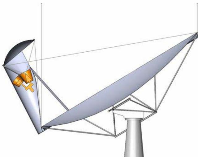
**Figure 1. Offset Gregorian reflector model (Cornell-TDP)**
